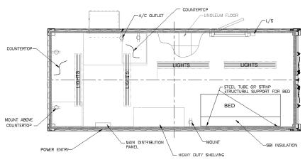
PLAN VIEW, ROOF REMOVED
