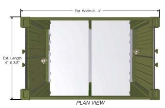
(4) Quadcon Containers coupled together to form (1) 20' ISO Module
