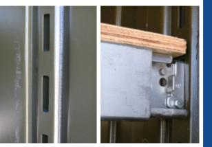
Shoring & Decking Beam engages on vertical "E" track system on ISO Container wall
