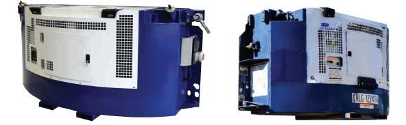
The "Clip On" Generator Set is designed to clip on to the front frame of a refrigerated container. The water cooled diesel generator can provide continuous (single voltage) electrical power to intermodal refrigerated containers. This unit is self contained with an integral fuel tank combined with engine, generator, battery and all operating controls.
