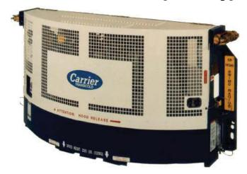
The "Clip On" Generator Set is designed to clip on to the front frame of a refrigerated container. The water cooled diesel generator can provide continuous (single voltage) electrical power to intermodal refrigerated containers. This unit is self contained with an integral fuel tank combined with engine, generator, battery and all operating controls.
