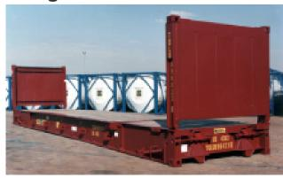
This is a heavy duty flatrack where the end walls fold flush with the floor. Four units fold into 8ft6in. This is one of 20 patent designs exclusive to CSA licensees.
