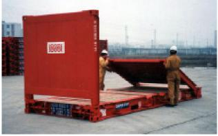
The end walls fold flush with the floor. Seven units fold into 8ft6in. This is one of 20 patent designs exclusive to CSA licensees.
