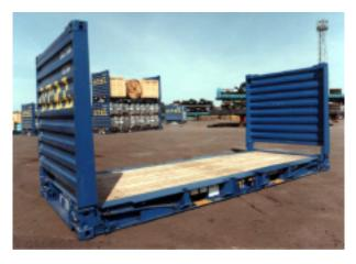
This flatrack benefits from a full width cargo deck, platform flat use when folded and high cube. In the commercial market it is a popular model. The corrugated steel end walls lie directly on top of the floor to become load bearing. Thus it can be used as a platform flat for long cargos such as pipes or sawn timber. Internal height is better than a Type (4) and seven units fold into 8ft 6in. This is one of 20 patent designs exclusive to CSA licensees.
